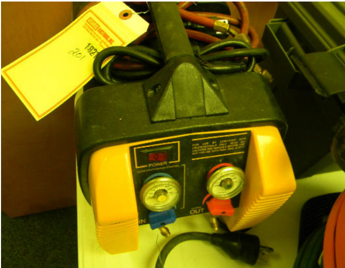
Lot #201 ~ 1 Appion G5 Twin cylinder - condensor for refrigerant recovery
